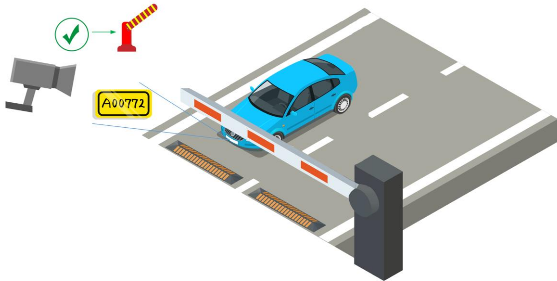
Figure 18-8 Example: Barrier Opened Automatically for Vehicle in Vehicle List
